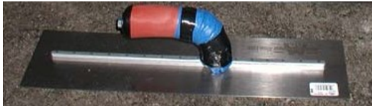
Photo 4 - Flat Trowel – Source: Tip Sheet: Concrete Trowel Handles – produced under CPWR Agreement #1020-005-56
